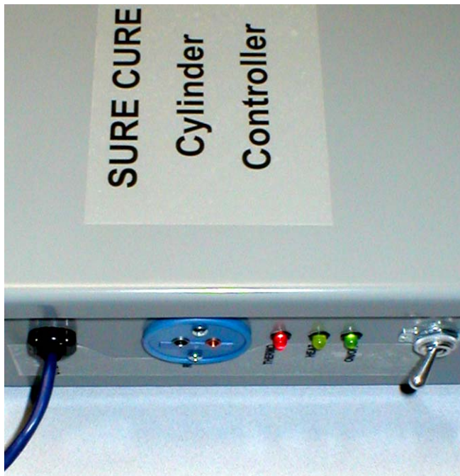
If the red light comes on and stays on, there is a problem with a thermocouple component.
