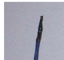
Complete thermocouple using shielded wire and electrical tape for electrical insulation
