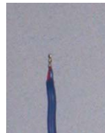
Soldered, twisted unshielded wire
