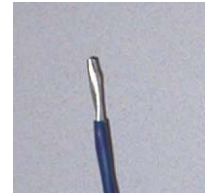
Shielded wire with outer insulation stripped
